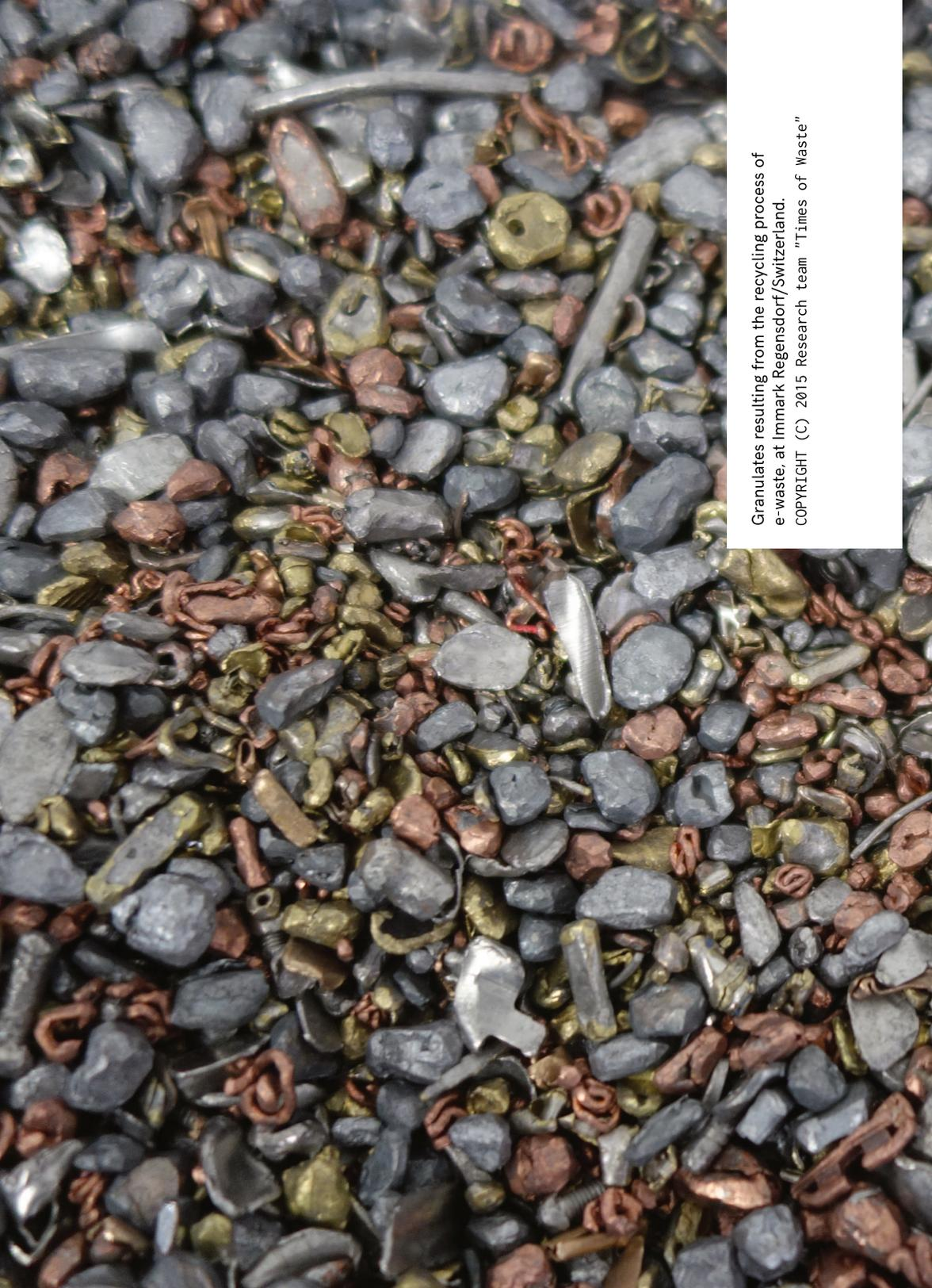
Granulates resulting from the recycling process of e-waste, at Immark Regensdorf/Switzerland.
